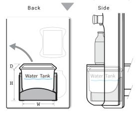
Removable Waste Water tank is supplied if option of drain pipe through the wall is not feasible. [manually empty water in period of time] Tank Capacity: 1 L
